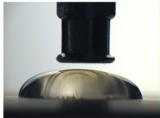
Fig. 2. The sessile drop on the brass plate and the benchmark of a linear dimension above it.
